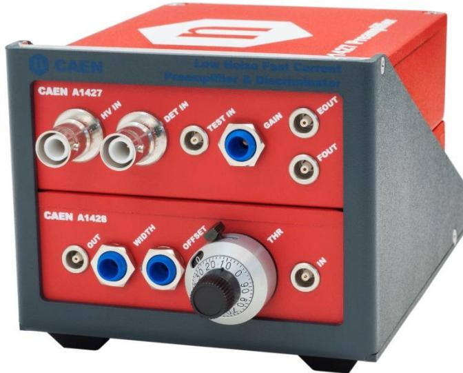
The A1427 is a fast and low noise current preamplifier with AC coupled input. It is suitable for fission chambers detectors and proton recoil counters.
