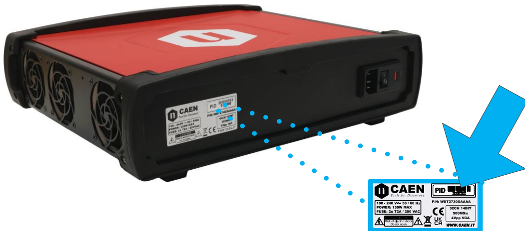
Fig. 4.2:PID location on Desktop Digitizer (the number in the picture is purely indicative)
