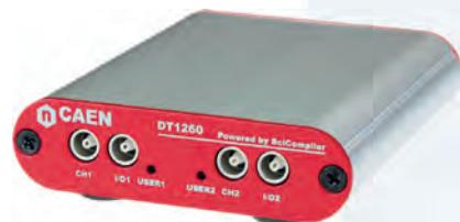
The kit allows to develop both FPGA firmware for custom digital pulse processing and software application for data readout, using the generated libraries.
