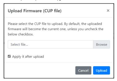
Before the firmware upload process begins, a message will appear warning the user that the transceiver currently in use on the board is incompatible with the selected firmware. The firmware will be set as the default and will take effect after the next reboot. Be sure to replace the transceiver while the device is powered off.
