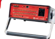
R5560SE 128 Ch.14 bit 125 MS/s Digitizer with single-ended inputs
