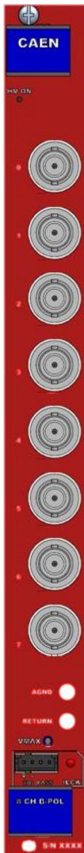
**HV Output 0..7:** Radiall SHVR317580 connector; HV channel output.
