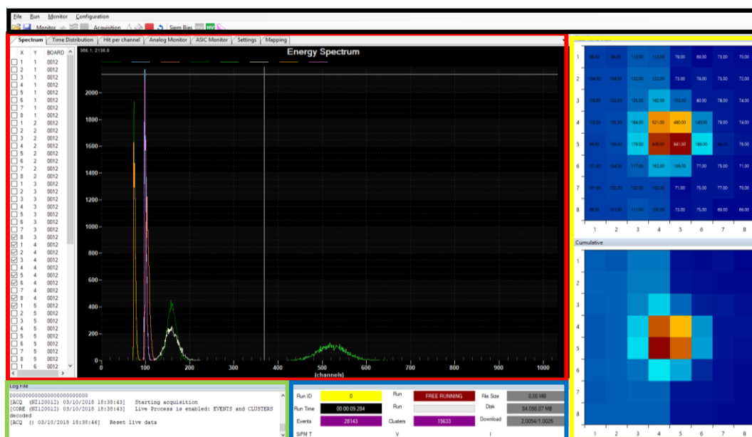
Figure 15.2: the main window of the DT5550W Readout Software. The main areas are highlighted. Black: menu and control toolbar. Red: main working area. Yellow: event display area. Green: log area. Blue: DAQ status.
