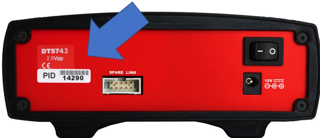
Fig. 5.1: PID location on DT5743 (the number in the picture is purely indicative)
