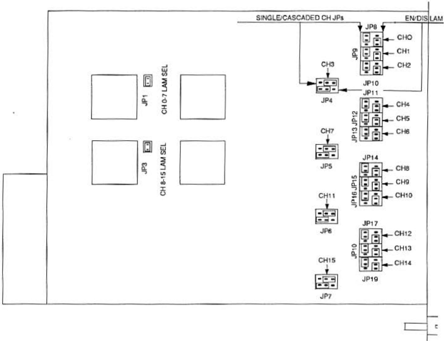
The module comes from CAEN with the internal jumpers configured as shown in figure above.
