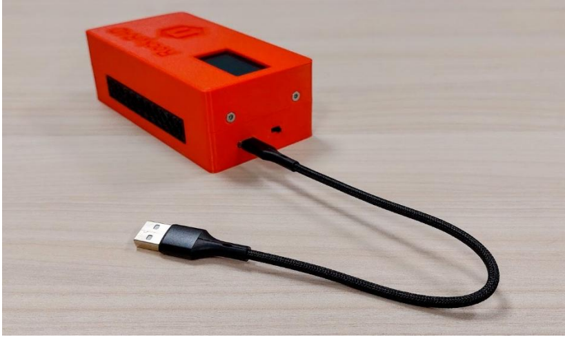
Fig. 5.1: Power supply cord connected to SP5660.
