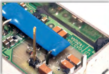
Fig. 1: Special materials and layout have been adopted to minimize possible issues due to thermal expansions
