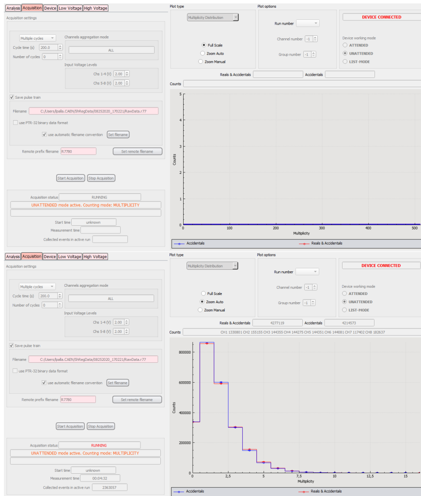
Fig. 2.5: The CAEN NCC GUI provided for a Guest (top) and for a User (bottom). In case of a Guest access, the acquisition status is shown on the Acquisition status section, but the collected data are not visible.
