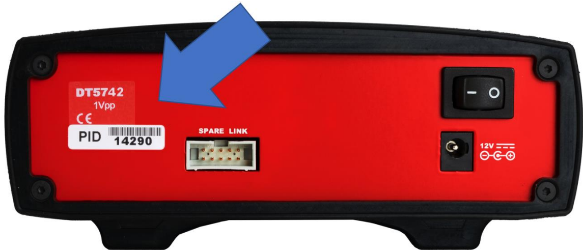
Fig. 5.1: PID location on the Desktop device (the number and digitizer model in the pictures are purely indicative)
