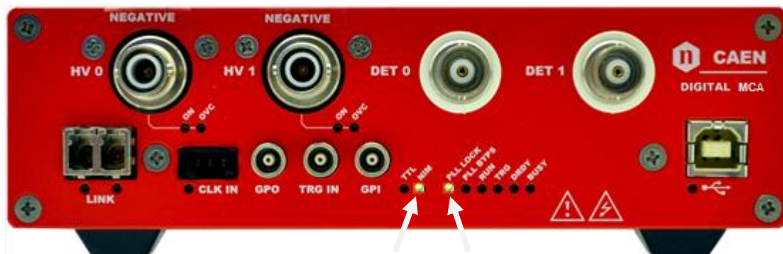
Fig. 10.1: Front panel LEDs status at power-on
