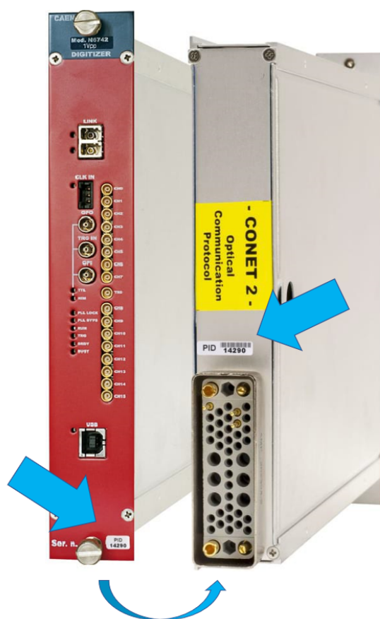
Fig. 5.1: PID location on NIM digitizers (the device model and the number in the picture are purely indicative).
