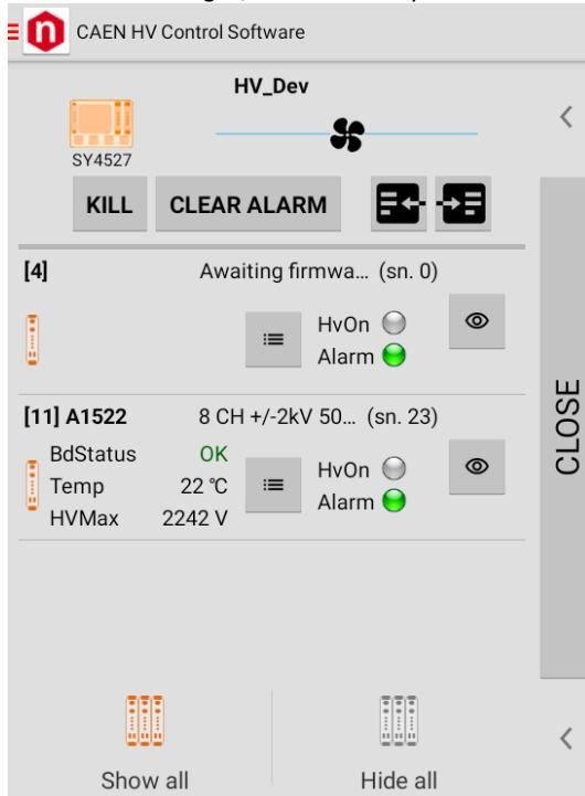
System Home shows what types of boards are inserted into the crate and in which slot they are plugged into, between [ ]. A short description of the board model follows with its features, serial number, and firmware release.
