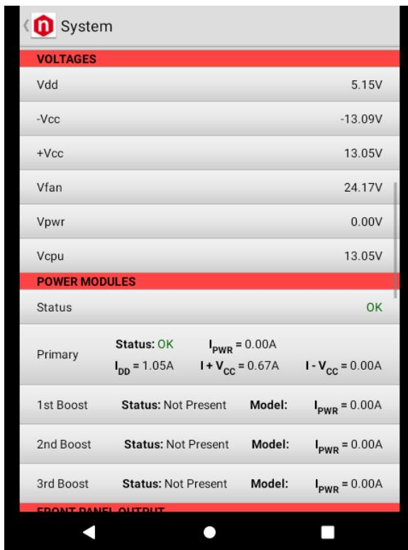
This option allows to monitor the voltage status of primary and booster power supplies
