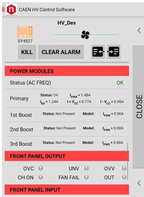
This option allows to monitor the front panel output status
