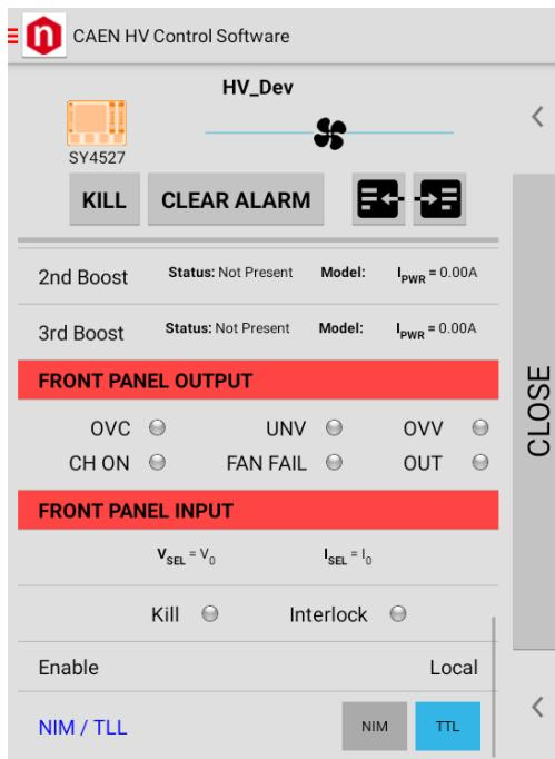
This option allows to monitor the front panel input status
