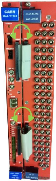
Figure 10.3: Connection of the V1741 to the A746B 64-ch LEMO adapter
