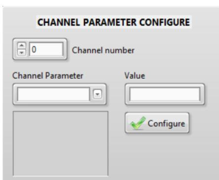
Select the Channel number and parameter, then enter the set value and confirm with "Configure".
