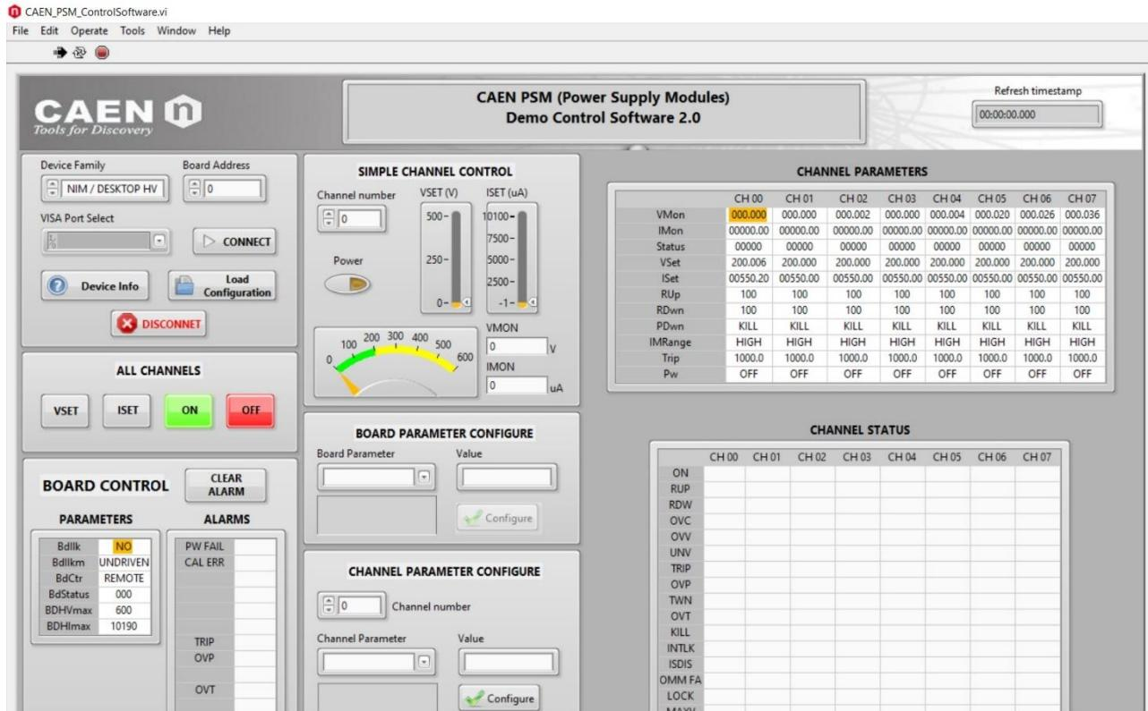
Select the Board to communicate with, by setting the board family and board address (if present), then confirm with [CONNECT] in the **Connection** box:
