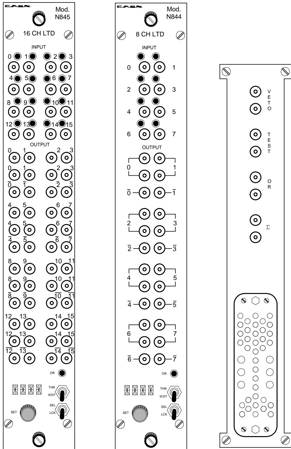
Fig. 2.1: Mod. N845-N844 front panel and back panel
