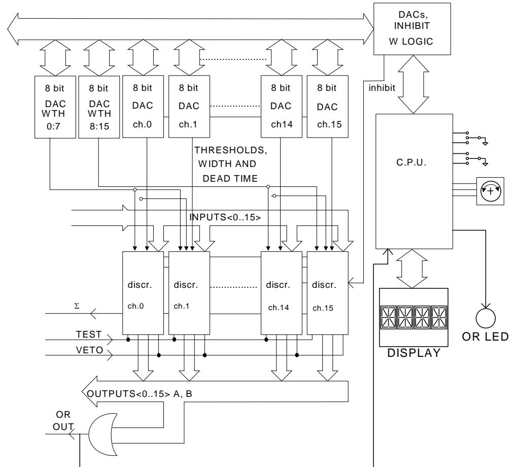
Fig. 1.1: Mod. N845 Block Diagram (16 Channel)
