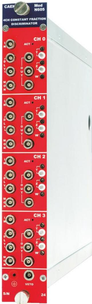
The N605 houses four independent 20% Constant Fraction Discriminators (CFD) in 1-unit wide NIM. The module is intended for high resolution time measurements, where fast signals with rise time as low as 0.8 ns are involved. Those may involve the use of radiation detectors made of fast scintillators, PMT, microchannel plates and fast semiconductor detectors.
