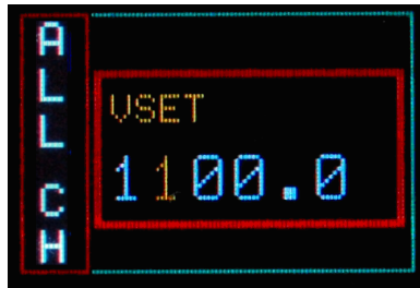
Fig. 3.23: Group Channel VSET digit access screen
