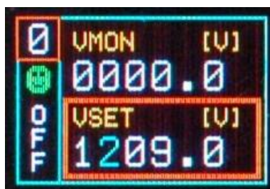
Fig. 4.14: Channel VSET digit confirm screen
