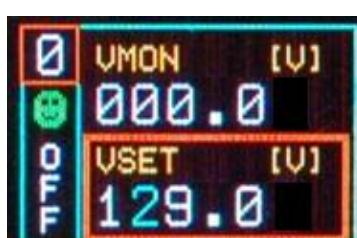
Once all the digits are set to the desired value, turn the TUNE ROTARY SWITCH until the parameter name returns blue
