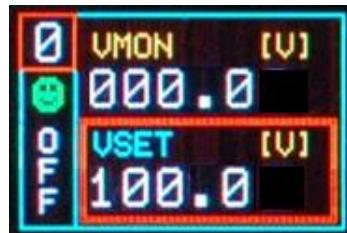
Turn the TUNE ROTARY SWITCH until the value digit to be edited is shown in blue, the parameter name in yellow
