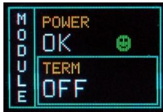
Push the TUNE ROTARY SWITCH in order to access MODULE parameters; the MODULE frame becomes red:
