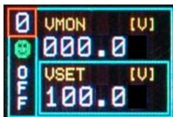
Push the TUNE ROTARY SWITCH: at this point the parameter is selected, its frame is shown in red and its name in blue; it is now possible to change the parameters value
