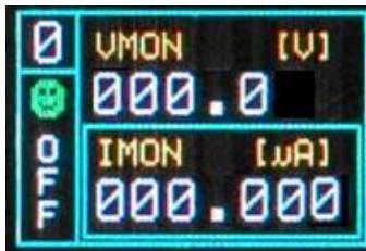
now connect the HV cable linking the outputs to the loads to be supplied and enable the HV outputs switching the HV\_EN/OFF/KILL 3 POS. SWITCH in the HV\_EN position; the Display will show the following message in the left lower row:
