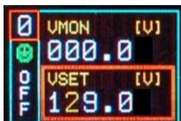
Confirm it by pushing the TUNE ROTARY SWITCH, the edited digit returns blue
