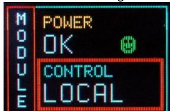
Select the desired value by turning the TUNE ROTARY SWITCH and confirm it by pushing the switch itself.
