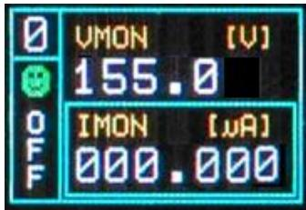
The KILL position of the HV\_EN/OFF/KILL 3 POS. SWITCH allows to turn off the module at the fastest available rate; the Display will show the following message in the left lower row:
