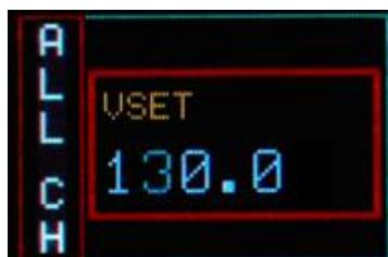
Once all the digits are set to the desired value, turn the TUNE ROTARY SWITCH until the parameter name returns blue. Push the TUNE ROTARY SWITCH in order to de-select the parameter, the frame returns to blue; when the parameter is not active, the parameter status of the four channels is shown.
