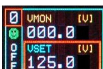
Push the TUNE ROTARY SWITCH in order to de-select the parameter, the frame returns to blue
