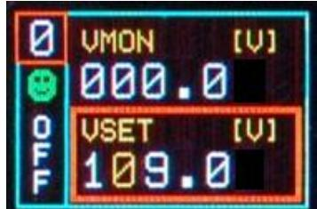
Turn the TUNE ROTARY SWITCH until the digit reaches the desired value
