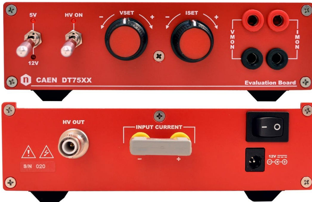
Fig.2: DT75xx front and rear panel
