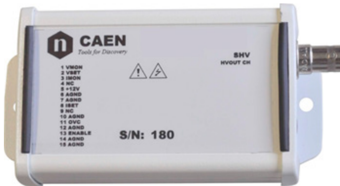
Fig. 7: A7520NB connector pin description
