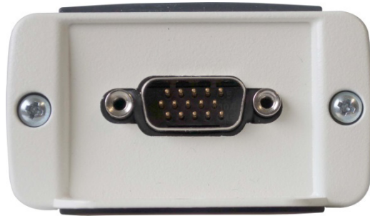
Fig. 6: A7520xB Back panel with 15 Pin Male High Density D-Sub Connector
