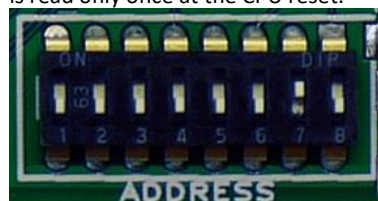
Figure 9.10: the 8-bits MAC address switch array. The configuration shown in the picture [01000000] corresponds to MAC[5] = 0X40.
