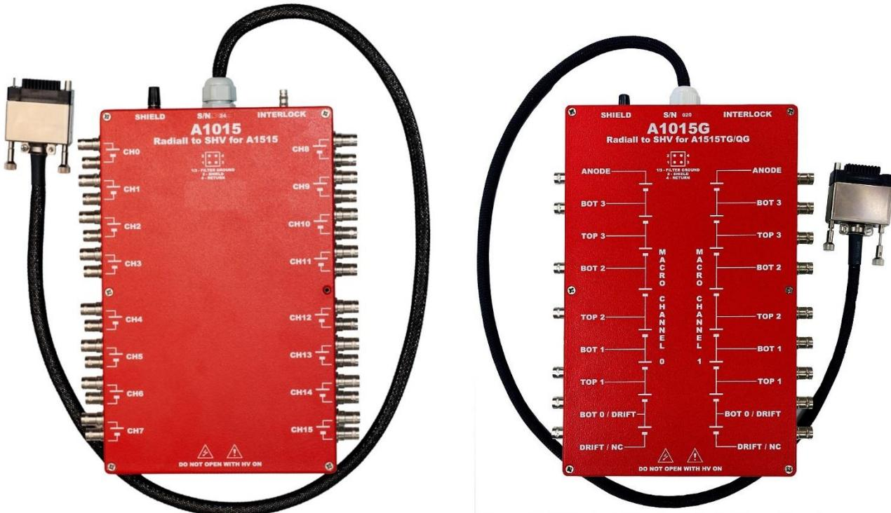
The CAEN A1015G is a 14/16 Stacked Channel Multipin Radiall to SHV connector Adapter for the A1515TG and A1515QG power supply modules; it allows to adapt the Radiall 691803004 type Multipin connector into Radiall SHV R317580-type HV coaxial connectors. Moreover, it is possible to configure the output stages with a RC filter. Please check the internal settings before each use.
