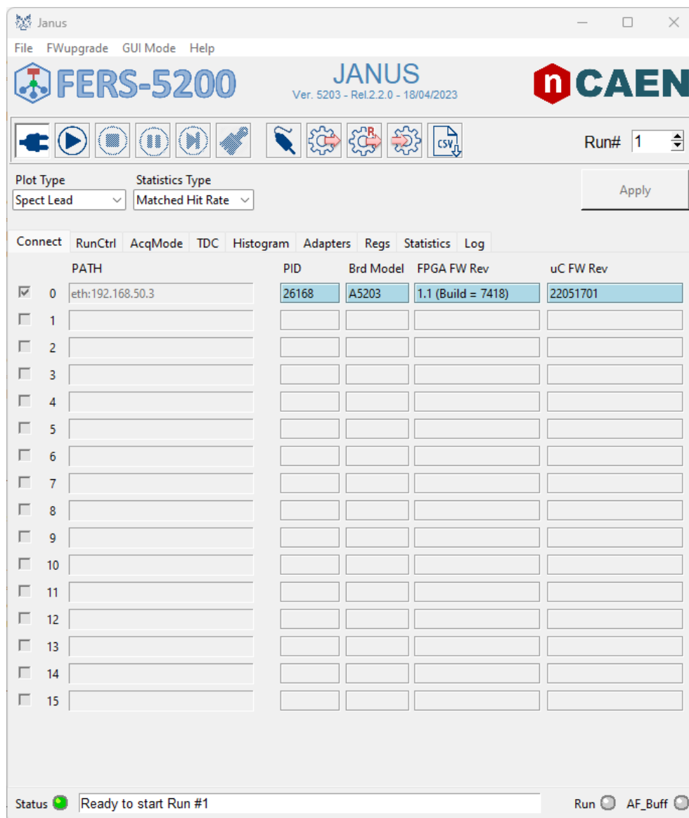
Fig. 3.15: Janus 5203 interface when the connection is established.
