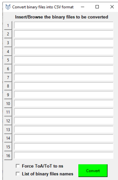
Fig. 3.8: Binary to CSV converter window.
