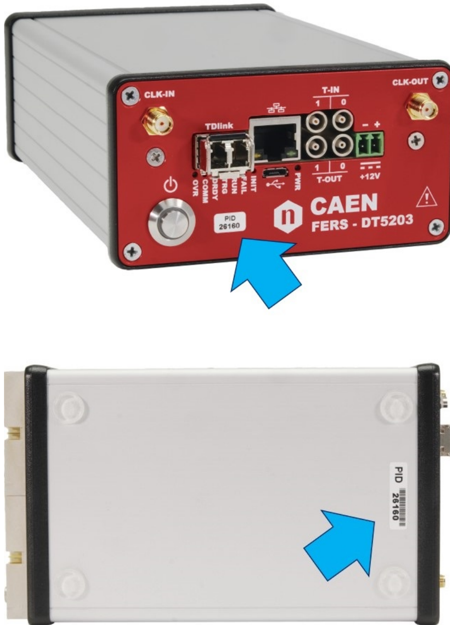
Fig. 5.2: PID location on DT5203 (the number in the picture is purely indicative) on the front panel of the board ( top ) and on the bottom side ( bottom ).
