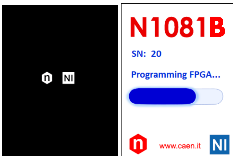
Figure 12.2: the touchscreen display of the N1081B during boot process (left) and programming process (right).
