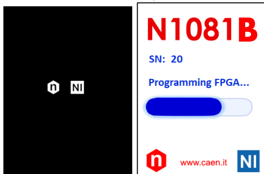
Figure 14.1: the touchscreen display of the N1081B during boot process (left) and programming process (right).
