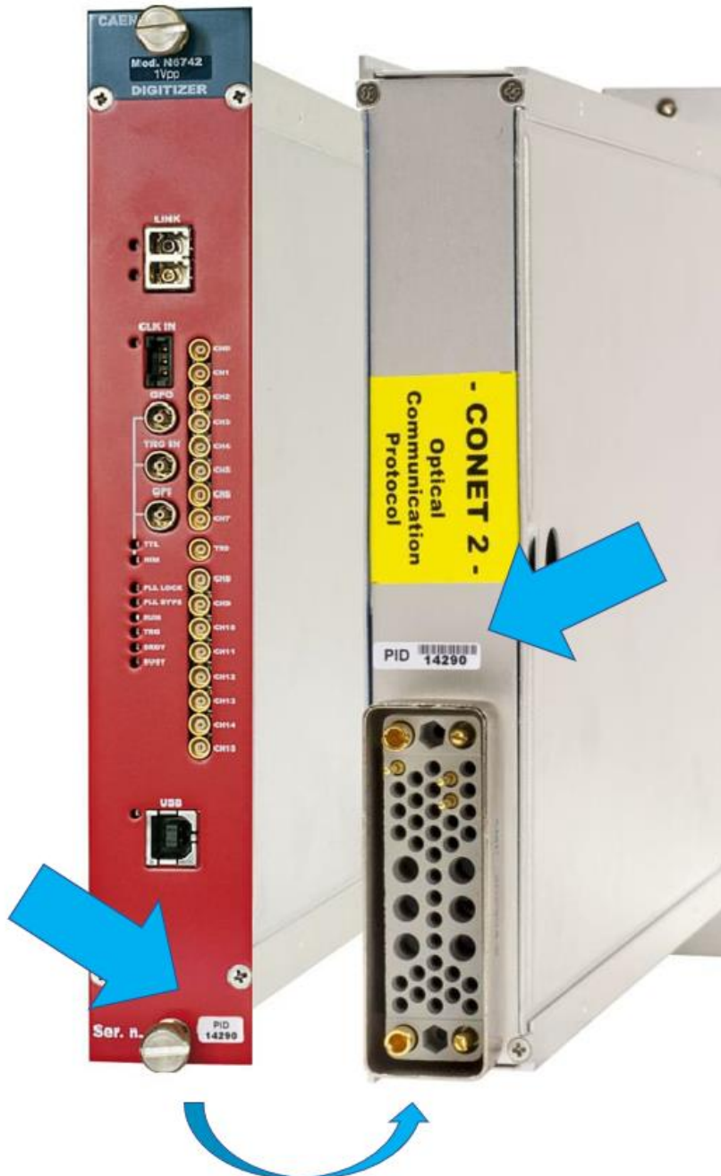
Figure 5.1: PID location on the Desktop device (the number and digitizer model in the pictures are purely indicative)
