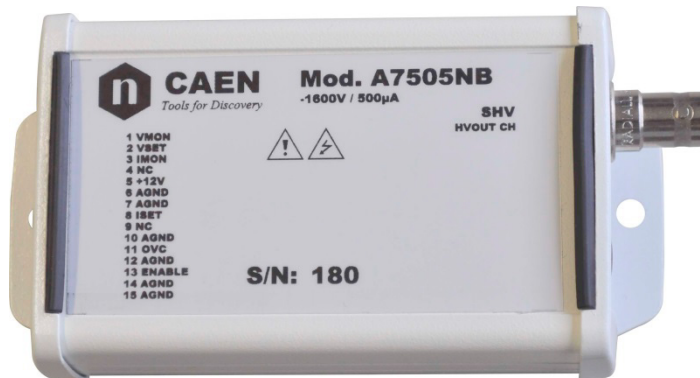
Fig. 13: Mod. A7505NB connector pin description
