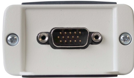
Fig. 12: A7505xB Back panel with 15 Pin Male High Density D-Sub Connector
