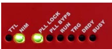
Fig. 11.1: Front panel LEDs status at power-on.
