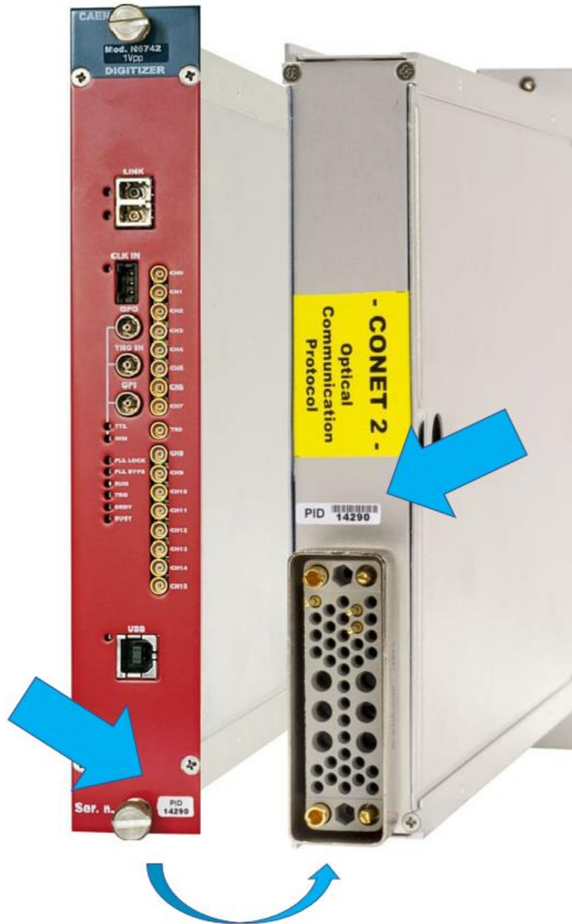
Fig. 4.1: PID location on the NIM device (the number and digitizer model in the picture are purely indicative)
