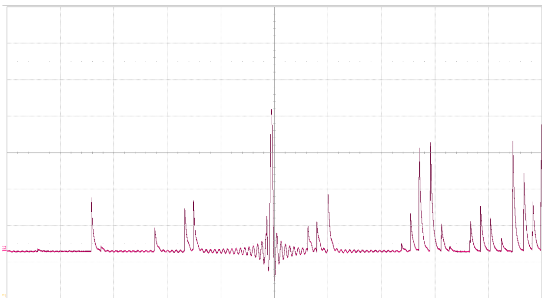
Fig. 6.21: Analog output signal with artificial interference.
