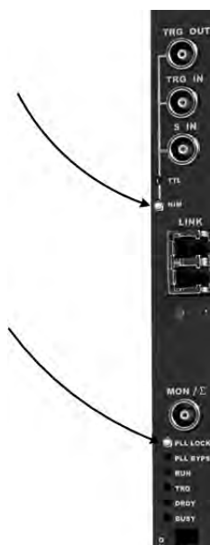
Fig. 10.1: Front panel LEDs status at power-on.
