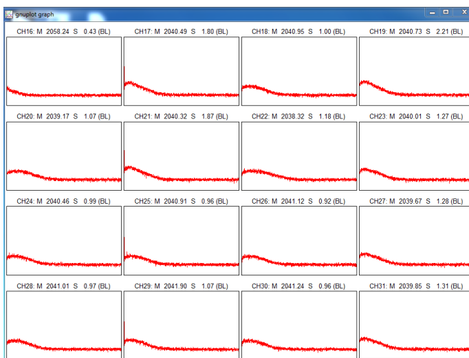
Fig. 6.8: 16-channel FFT plot by gnuplot utility
