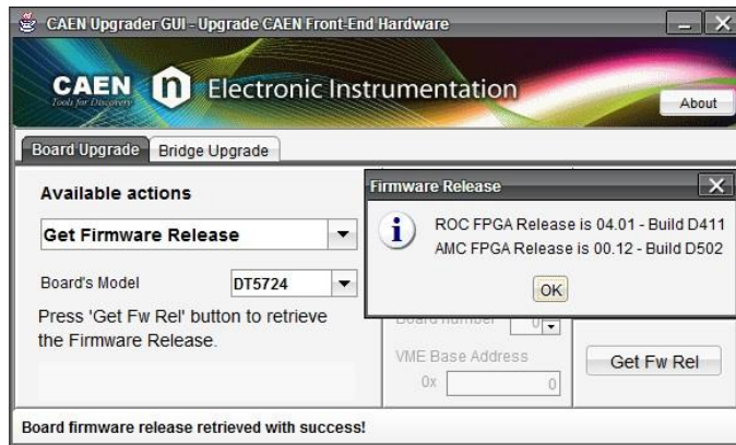
Fig. 1.1.1: The Get Firmware Release option of CAENUpgrader
