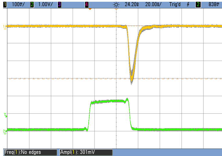
Figure 2: Oscilloscope view of the UV-LED signal from PMT (yellow), and its synchronization signal (green).
