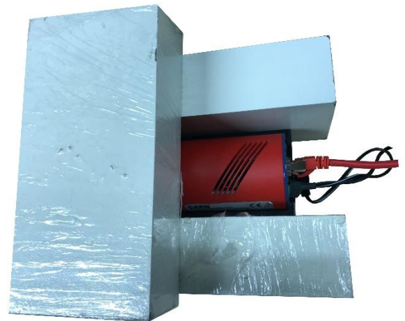
Experimental setup block with Lead blocks covering the active scintillator of i-Spector digital.
