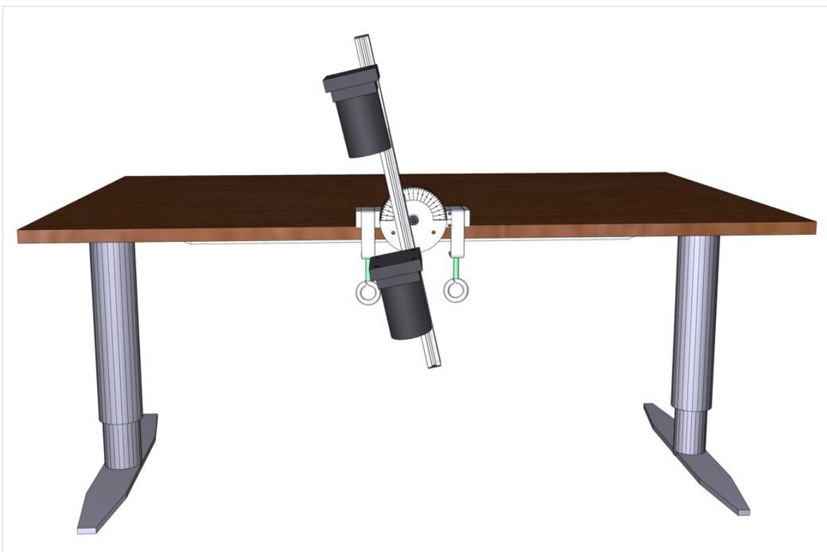
Fig. 2.2: Muons telescope (SP5608 based).
