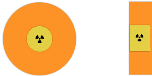
Fig. A.2: The top and side view of the ^{22}\text{Na} source scheme (not to scale): the radioactive liquid (yellow) is encapsulated into a plastic enclosure (orange) with a sharp edge on the left and a smoothed edge on the right
