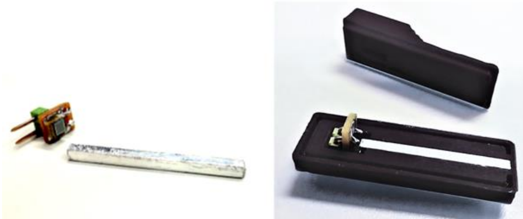
Fig. 8.4: LYSO crystals 2 \times 2 \times 30 \text{ mm}^3 by Kinheng Crystal and 1 \times 1 \text{ mm}^2 MPPC (S10362-11-050P) produced by HAMAMATSU Photonics. On the right side, The EasyPET light-tight case with the housing for the scintillating crystal and the SiPM sensor
