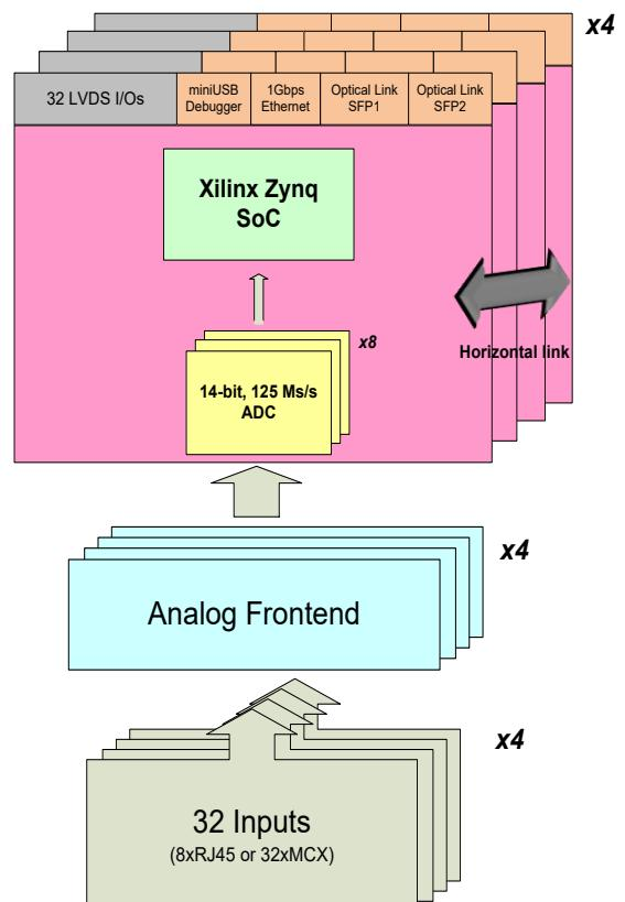
**R5560SE is suitable for building an integrated multi-channel DAQ system for Position-Sensitive Detectors, Gaseous Detectors, PMTs, Germanium detectors, RPCs and other detectors.**
