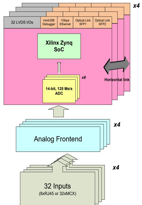
**R5560 is suitable for building an integrated multi-channel DAQ system for Position-Sensitive Detectors, Gaseous Detectors, PMTs, Germanium detectors, RPCs and other detectors.**
