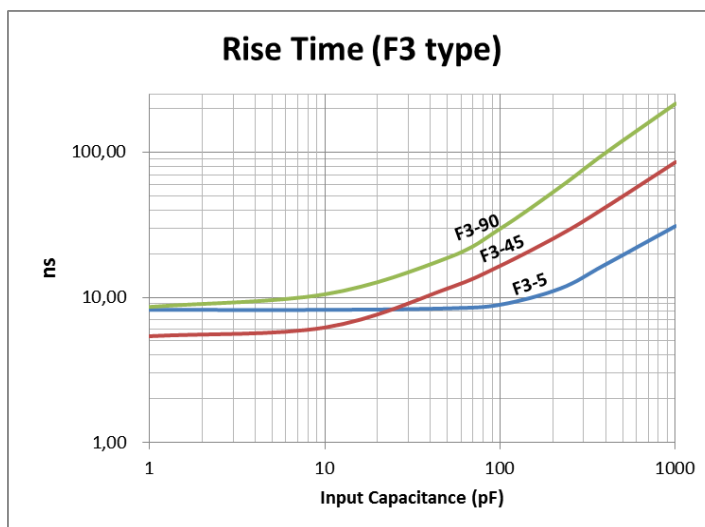
Fig. 1 : Typical Rise Time vs input Capacitance (test input rise time = 1.6 ns, amplitude: 200 mV, 50 \Omega termination)
