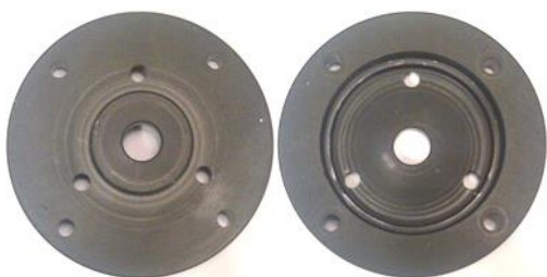
Fig.4: Front and Back views of the internal PVC holder
