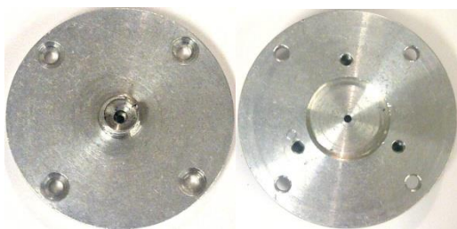
Fig.2: Front and Back view of the external aluminum holder
