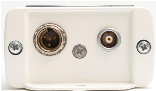
Fig. 4.1: A7501PB Front panel, LEMO HV and 4-pin Mini XLR connectors for Auger IMON and temperature remote inputs
