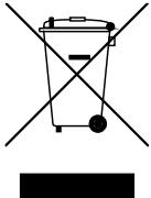
The crossed bin symbol indicates that the device shall not be disposed with regular residual waste.
