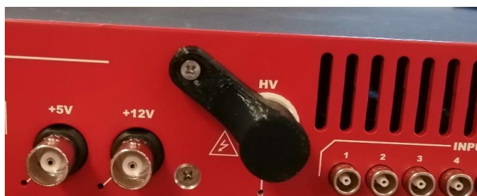
Fig. 5.5: SHV safety cap
