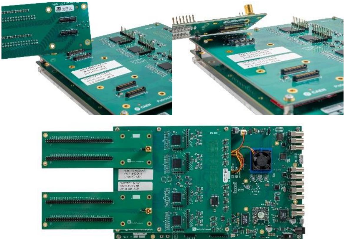
Figure 10.7: Top: how to plug the pitch adapter on the board's SiPM connector. The connectors are pressure-pluggable. Bottom: general view of a DT5550W with A55CIT4 piggyback and two pitch adapters plugged in. In this configuration, all 128 channels of the DT5550W board are exposed on the strip connectors.
